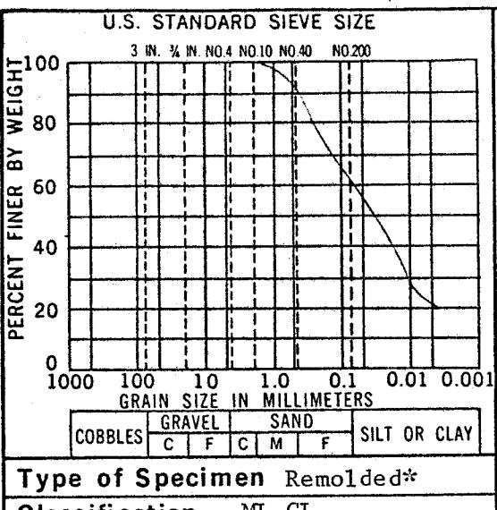
Type of Specimen Remolded\*
